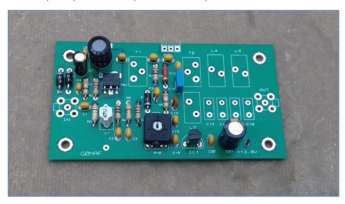
In the picture above, the only components remaining to be fitted are L3, the 2 transformers and a low pass filter for the band of choice. Winding and fitting the transformers T1 and T2 needs concentration while winding L4 and L5 needs patience. If you want a break from soldering, this is a good time!
