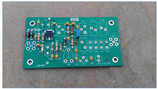
In the picture above you may spot that I have fitted a 1mm terminal pin for the supply connection. After trying a couple of different techniques I have concluded that a stranded wire is probably the best method of getting power to the board. So, leave this pad until it's time to test the board, then solder on a length of wire.
