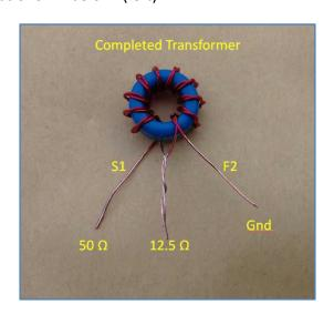
Next, strip the enamel from S2 and F1, taking care not to damage the wire if you use a knife. Then loosely twist S2 and F1 together. This is the low impedance (12.5 ohm) side of our broadband RF transformer. The connections are shown above (right). - Don't mix them up !!!
